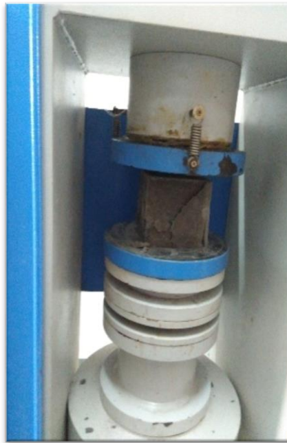
Fig 9. Testing of cube
