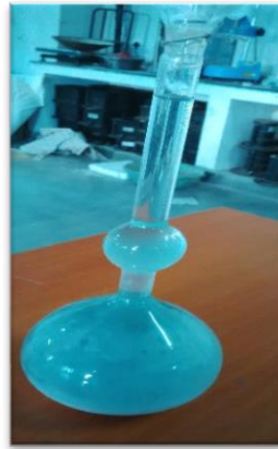
Fig 1. Le Chatlier flask (specific gravity of ESP)
