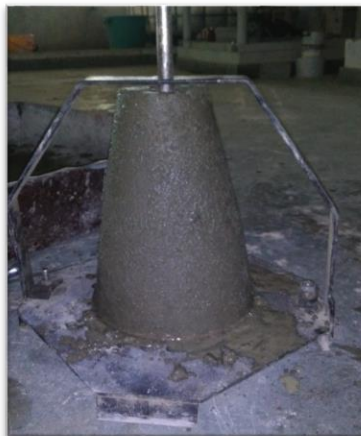
Fig 16. Shape of slump (true slump)
