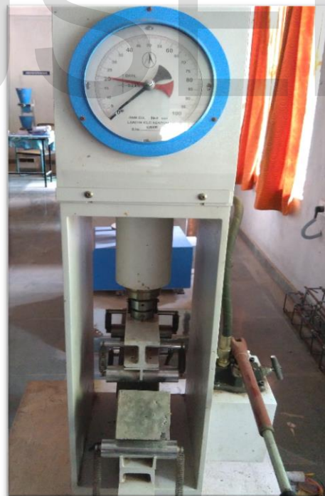
Fig 11. Testing of flextural strength
